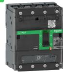
Circuit breaker, ComPacT NSXm 100F, 36kA/415VAC, 4 poles 4D (neutral fully protected), TMD trip unit 100A, lugs/busbars
